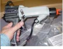
The unique fast-set aliphatic and aromatic products are delivered through commercially available proportioners feeding commercial and proprietary spray guns. The proprietary formulated components are electrically charged with specialized generators designed specifically for plural component use. Initial gel times can be adjusted from five seconds to several minutes. Dry to touch times are less than a minute for the fast-set systems and are proportionate for the slower systems.
